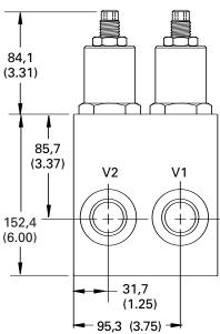
The MCV4-16 is a dual inline housing type motion control or load holding valve. This valve controls a moving load and prevents loads from running ahead of a pump. It will also lock or hold a load in any position and provides for thermal expansion relief and make-up oil.
